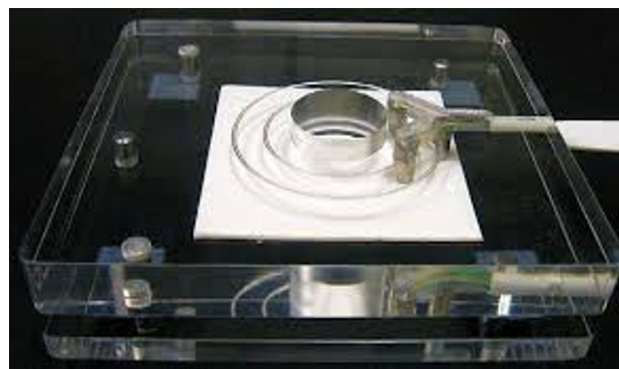
Figura 2. Capillary Suction Timer da Fann.
