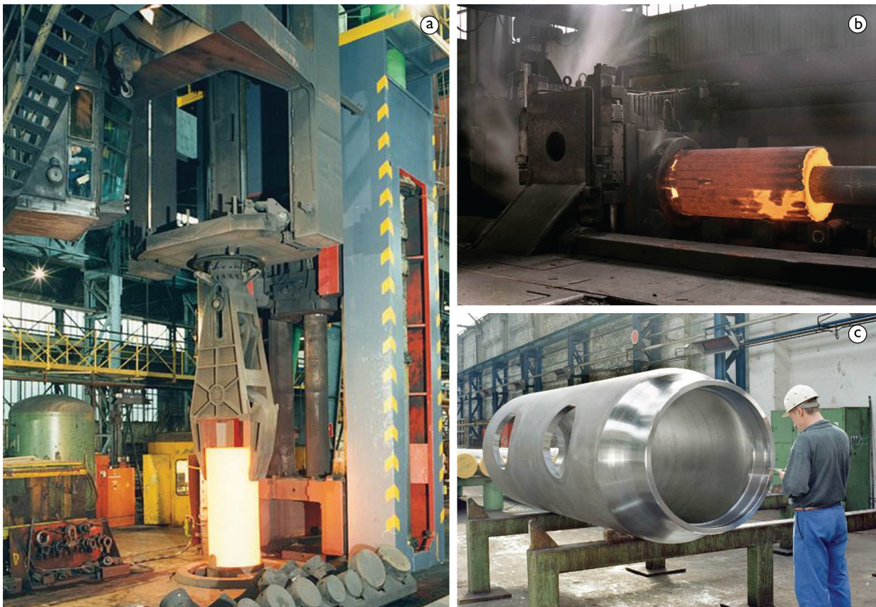
Figure 2. Manufacturing of tubular goods in the Vallourec Reisholz mill according to the Ehrhardt process: (a) piercing, (b) drawing, (c) final product [1].
