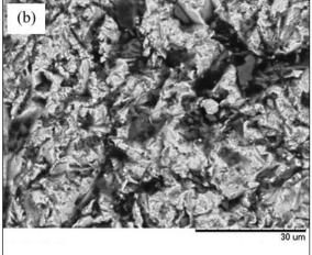
**Figure 3.** Abrasive wear modes: (a) "grooving abrasion" [3,12] and (b) "rolling abrasion".
