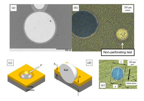
**Figure 2.** Examples of wear craters generated on coated systems: (a) multi-layer, (b) thin film of TiN (crater of right: non-perforating test, e.g., without reaching the substrate), (c) total wear volume – "V" (schematic illustration), (d) total crater depth – "h" and coating thickness – " $h_c$ " (schematic illustration), (e) internal diameter – "a" and external diameter – "b" [11].
