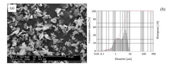
Figure 5. SiC abrasive [12]: (a) scanning electron micrograph and (b) particle size distribution.
