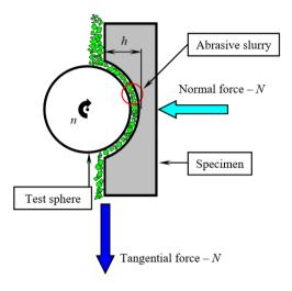
**Figure 1.** Micro-abrasive wear test by rotating ball: A representative figure showing the operating principle and the abrasive particles between the test sphere and the specimen; "h" is the depth of the wear crater and "n" is the test sphere rotational speed.
