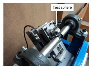
**Figure 4.** Ball-cratering micro-abrasive wear test equipment used in this work: free-ball mechanical configuration.
