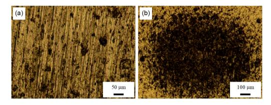
Figure 6. Occurrence of (a) "grooving abrasion" and (b) "rolling abrasion" on the surface of the thin films.
