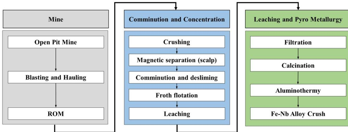
Figure 2. Fe-Nb alloy production flowsheet.
