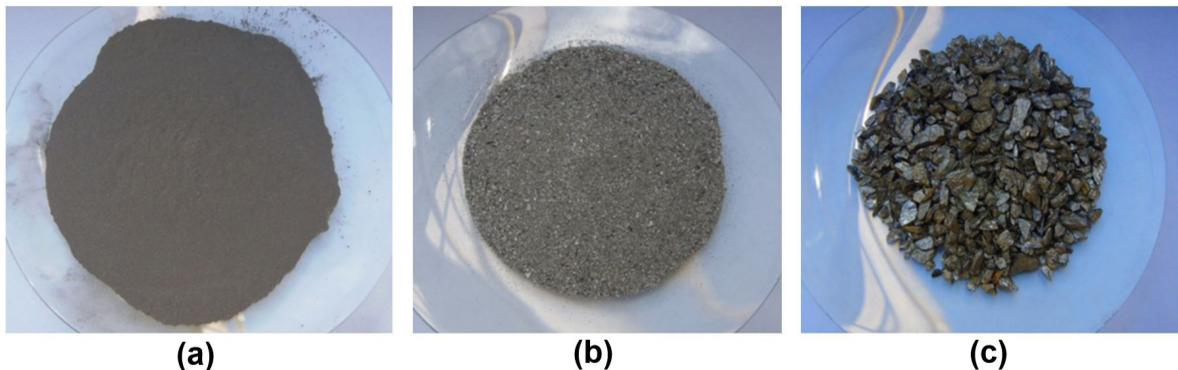
Figure 3. Fe-Nb fine particles: (a) under 2 mm (or type A), (b) between 1 and 5 mm or type B and (c) between 3 and 15 mm or type C.
