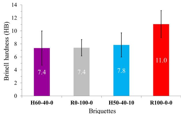
Figure 9. Briquettes average Brinell hardness.
