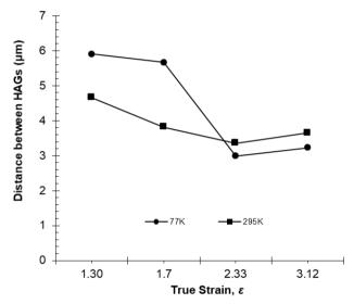
**Figure 3.** Distance between high-angle boundaries as a function of deformation.
