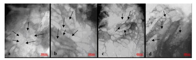
Figure 1. TEM micrographs of wires drawn at 295 K to diameters of (a) 5.00 mm ( $\epsilon$  = 1.30), (b) 4.14 mm ( $\epsilon$  = 1.68), (c) 3.15 ( $\epsilon$  = 2.23) and (d) 2.02 mm ( $\epsilon$  = 3.12).
