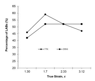
Figure 4. Percentage of low-angle boundaries as a function of deformation.
