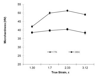
Figure 5. Vickers microhardness versus true strain for drawn wires processed at 295 K and 77 K.
