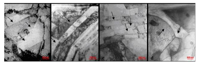
Figure 2. TEM micrographs of wiresdrawn at 77 K to diameters of (a) 5.00 mm ( $\epsilon = 1.30$ ), (b) 4.14 mm ( $\epsilon = 1.68$ ), (c) 3.15 ( $\epsilon = 2.23$ ) and (d) 2.02 mm ( $\epsilon = 3.12$ ).
