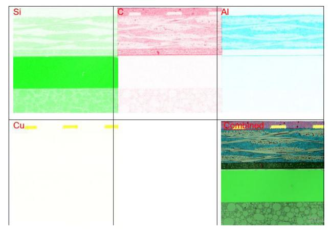
Figure 7. EDX images of the memory board, sampling B.
