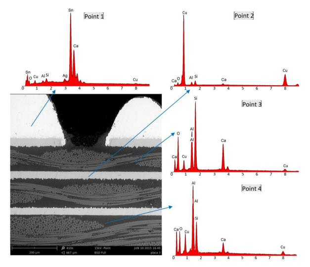
Figure 5. Image showing retro-scattered electrons of sampling A in the motherboard and the EDSs of points 1 (weld), 2 (copper track), 3 (glass fiber) and 4 (resin).
