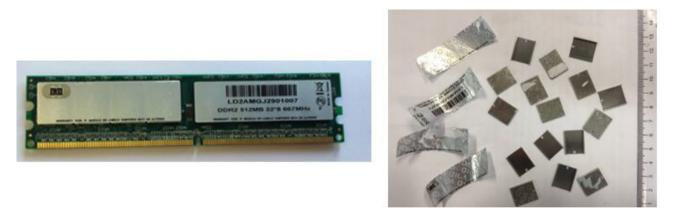
Figure 8. Memory board and components removed from it through manual dismantling.
