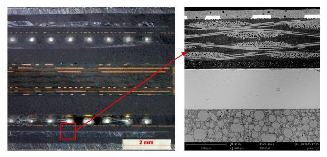
Figure 6. Image showing retro-scattered electrons of sampling B in the memory board. On the left, detail showing the region where the micrograph was analyzed.
