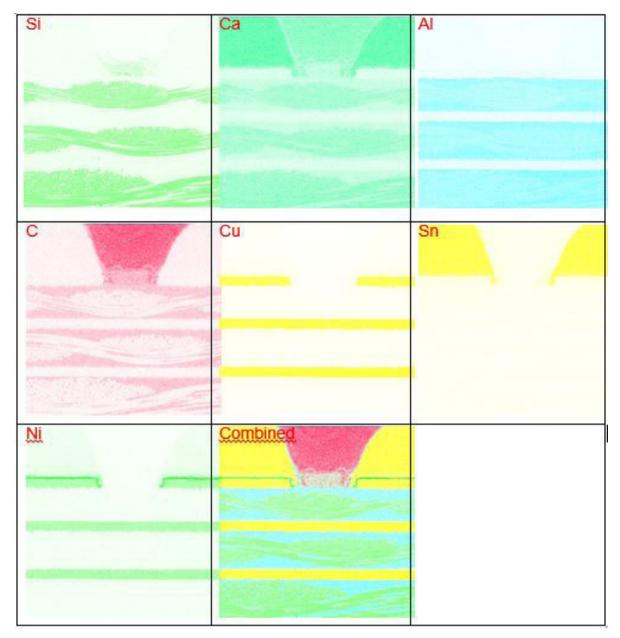
Figure 4. EDX images of the memory board, sampling A.
