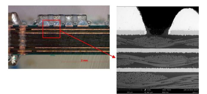
Figure 3. On the right, image showing retro-scattered electrons of sampling A in the memory board. On the left, detail showing the region where the micrograph was analyzed.
