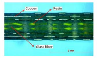
**Figure I.** Binocular microscope image showing the cross-section of the PCB-memory.
