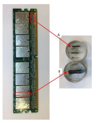
**Figure 2.** PCM-mem board with location of sampling points A and B, and identification of resin-embedded samples.
