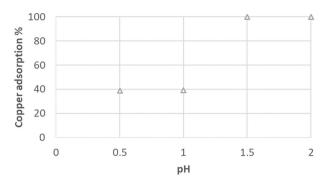
Figure 3. Percentage copper adsorbed for each pH studied in 120min, using 1g of resin, 50mL of solution at 25°C.  $\Delta$  = Percentage of copper ions adsorption.
