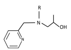
**Figure 1.** The hydroxypropyl-picolylamine functional group of Dowex XUS 43605 chelating resin [12].
