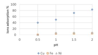
Figure 5. Percentage ions adsorbed for each pH studied in 120min, using 1g of resin, 50mL of solution at 25°C.
