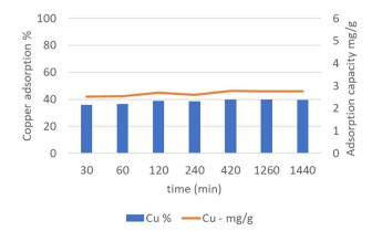
Figure 2. Percentage of copper ions adsorbed and adsorption capacity (mg/g) during the time (30-1440min) using 1g of resin, 50mL of solution and pH 0.5 at  $25^{\circ}$ C.
