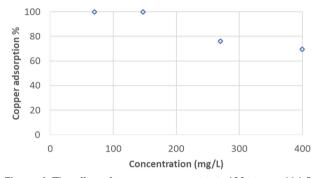
**Figure 4.** The effect of copper concentration in 120min, at pH 1.5, using 1g of resin and 50mL of solution at 25°C.  $\Diamond$  = Percentage of copper ions adsorption.
