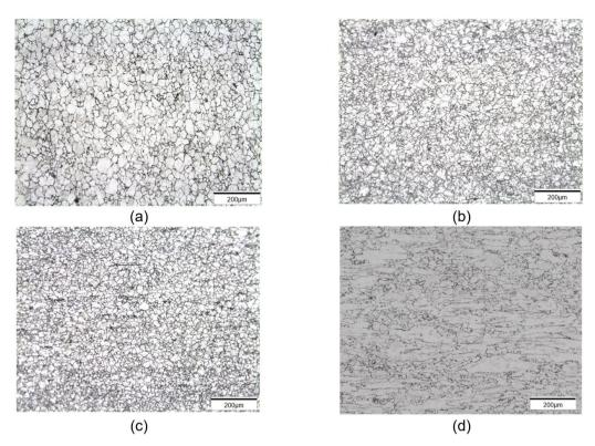
Figure 2. Austenitic grain size of longitudinal section of (a) mid-radius of Al-HR, (b) mid-radius Al-Nb-Ti-CR, (c) mid radius of Al-Nb-CR and (d) surface of Al-Nb-CR. Etched with aqueous solution of picric acid 2%.
