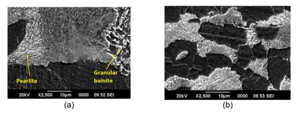
Figure 5. SEM micrographs of transversal section of (a) AI-HR and (b) AI-Nb-CR. Nital 2% etched.
