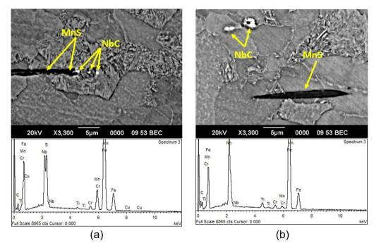
Figure 7. SEM and EDS analysis of coarse NbC and MnS precipitates. (a) AI-Nb-CR and (b) AI-Nb-Ti-CR. Nital 2% etched.
