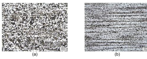
Figure 6. Microstructures of mid-radius longitudinal section of of (a) Al- HR, (b) Al-Nb-Ti-CR. Etched with Nital 2%.
