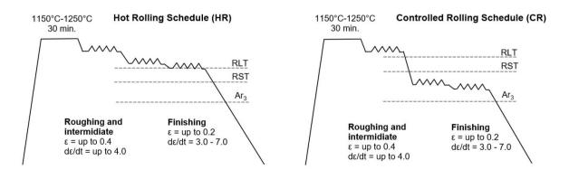
Figure 1. Hot rolling schedules used during rolling.
