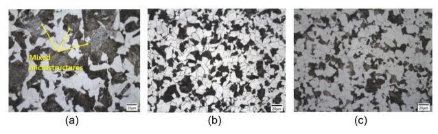
Figure 4. Microstructures of transversal section from Charpy samples tested in -40°C. (a) Al-HR, (b) Al-Nb-CR, (c) Al-Nb-Ti-CR. Nital 2% etched.
