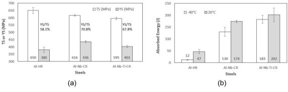
Figure 3. (a) Yield strength (YS), tensile strength (TS) and (b) absorbed energy (J).
