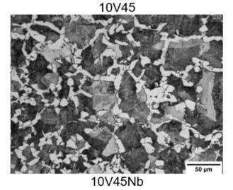
Figure 1. Light optical micrographs from the near-surface of the three industrially hot-rolled bars after air cooling [9,10]. 2% Nital etch.
