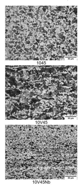
Figure 2. Near-surface microstructures of the three industrially thermomechanically rolled bars after air cooling [9,10]. 2% Nital etch.
