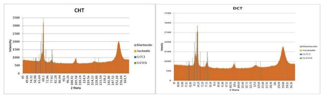
Figure 6. X-ray diffraction for CHT and DCT samples.
