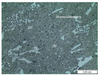
Figure 2. Micrography of CHT sample, where the martensite matrix, PC, SSC and LSC can be observed.
