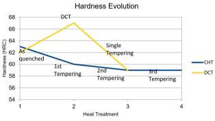
Figure 7. Hardness evolution after CHT and DCT.
