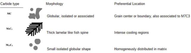
Figure 5. Carbides morphology and preferential regions in tool steels. Adapted from Vitry et al. [21]
