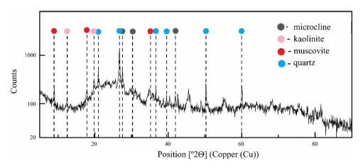
Figure 4. X-ray diffraction pattern of metakaolin (MK).
