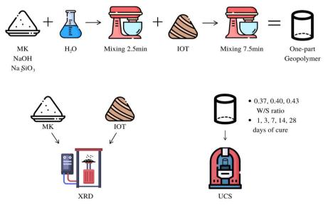
Figure 3. Experimental procedure.
