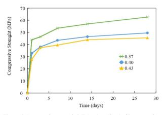
**Figure 6.** Compressive strength (MPa) x time (days) of 3 tests varying W/S ratio.
