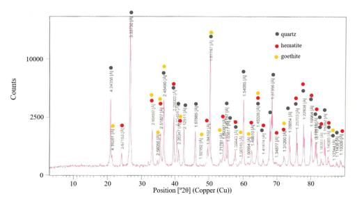
Figure 5. X-ray diffraction pattern of iron ore tailings (IOT).
