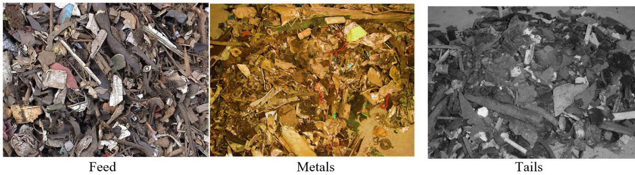
Figure 8. Metals separation via inductive sensing [2].
