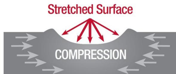
**Figure 6.** Schematic illustration of the surface after shot peening [16].
