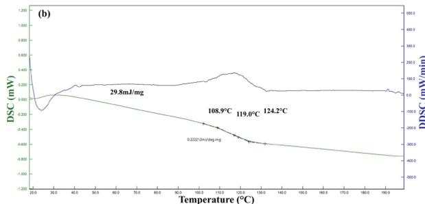
Figure 2. DSC curves of the neat epoxy resin: (a) first and (b) second heating runs.
