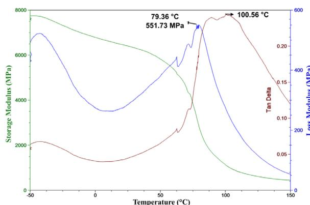
Figure 5. DMA curves for the storage modulus ( $E'$ ), loss modulus ( $E''$ ) and  $\tan \delta$  for the composites reinforced with 30 vol% of arapaima scales.
