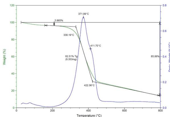
Figure 4. TGA and DTG curves for the composite reinforced with 30 vol% of arapaima scales.
