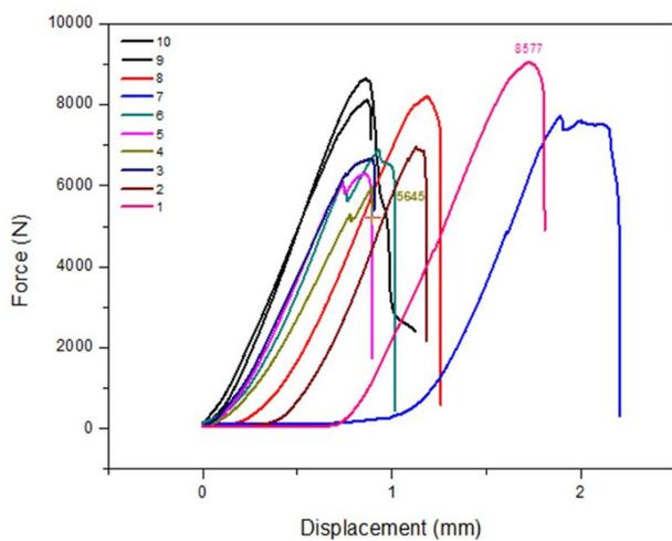
**Figure 6.** Force vs displacement curves from the compression tests of epoxy composites with 30 vol% of arapaima scales.
