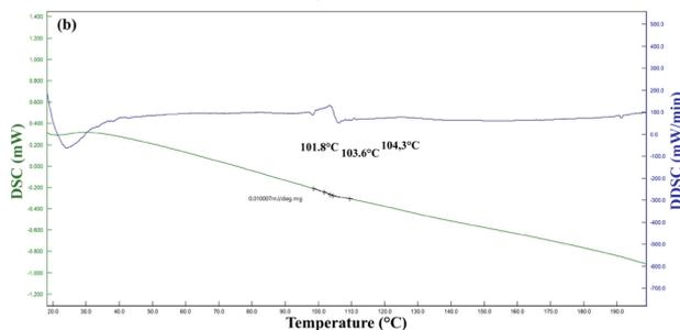
Figure 3. DSC curves of the 30 vol% arapaima scales reinforced composite: (a) first and (b) second heating runs.
