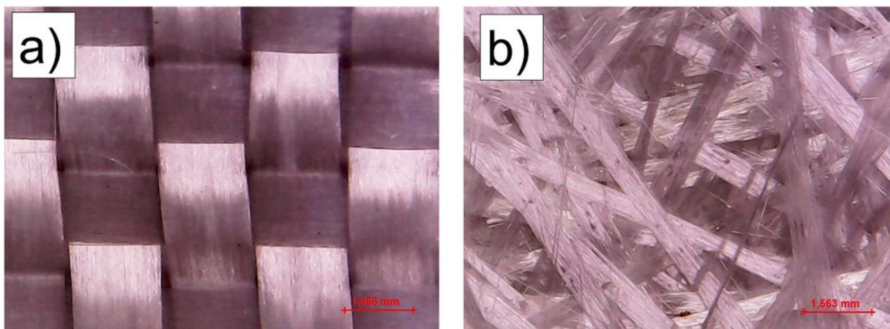
**Figure 1.** OM images of the surfaces of the (a) bidirectional fiberglass fabric and (b) multidirectional fiberglass blanket.
