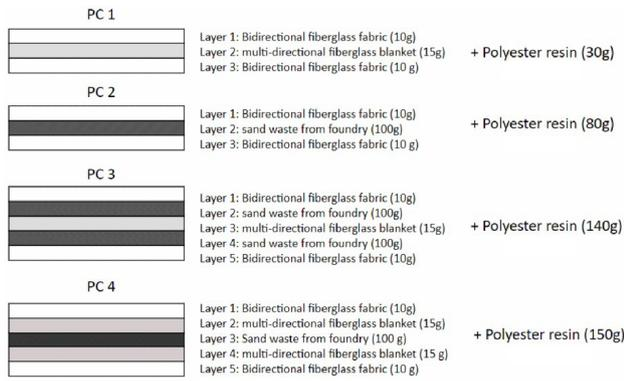
**Figure 2.** Identification and composition of the layers used for preparing the composites.
