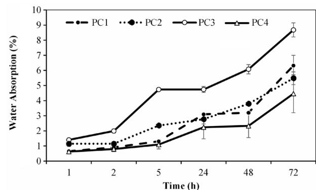
**Figure 5.** Water absorption of the composites with and without foundry sand.
