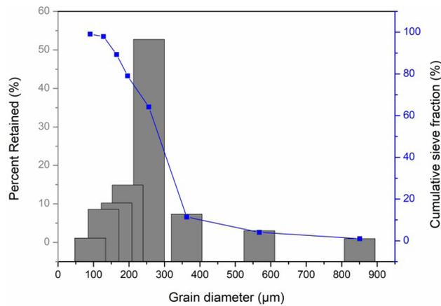
**Figure 4.** Granulometric analysis of foundry sand.
