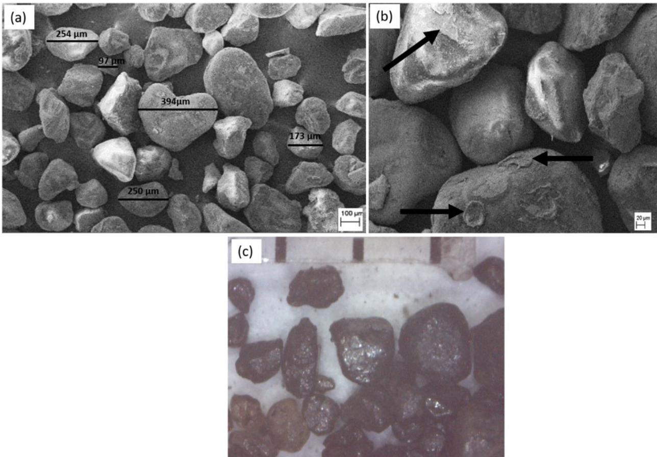
**Figure 3.** Micrographs obtained by the (a), (b) SEM and (c) OM of the sand discarded from the foundry process.
