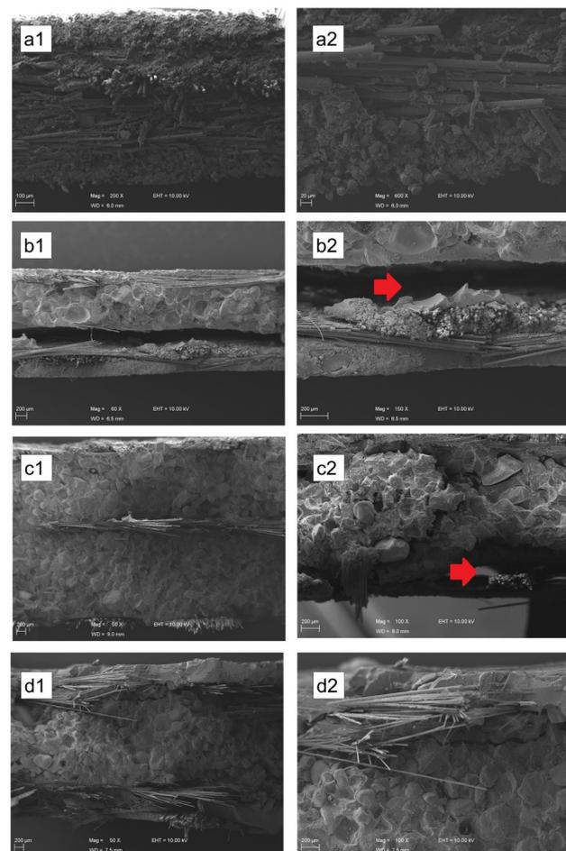
**Figure 6.** SEM micrographs, in the fracture region, after the tensile strength test of the sample (a) PC1; (b) PC2; (c) PC3 and (d) PC4.
