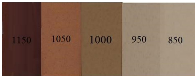
Figure 13. Color of the samples after ceramic firing at temperatures of 850 °C, 950 °C, 1000 °C, 1050 °C and 1150 °C.
