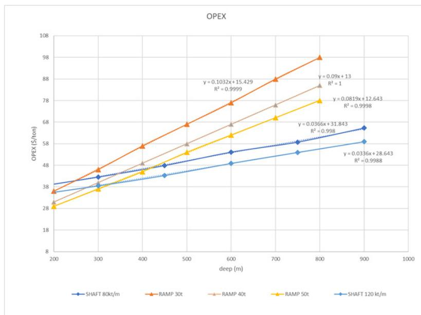
Figure 3. Opex for Ramp and Shaft adjusted for report of Rupprecht [11].
