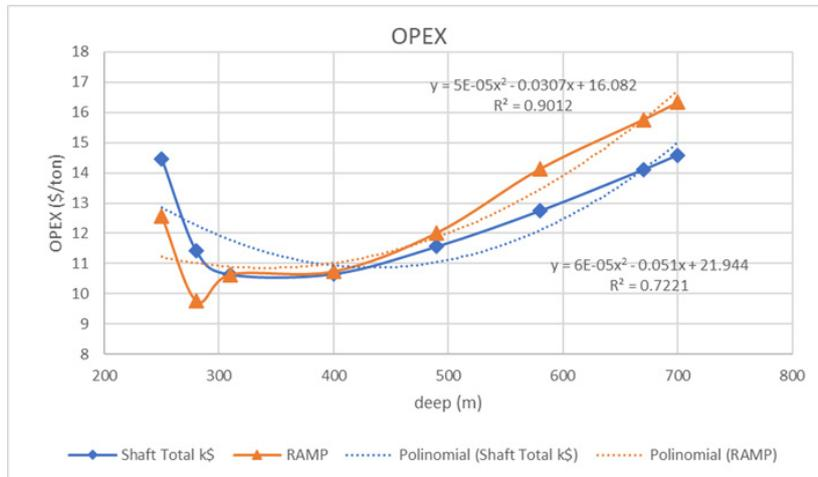
Figure 2. Opex for Shaft and Ramp adjusted for report of Elevli et al. [12].
