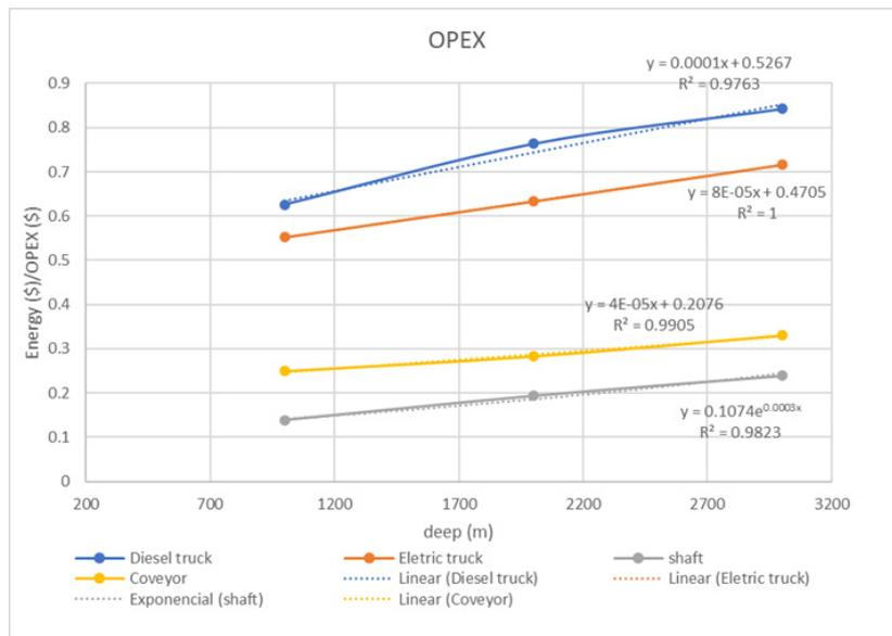
Figure 9. Relationship between Energy cost and transportation OpeX for Salama [4].
