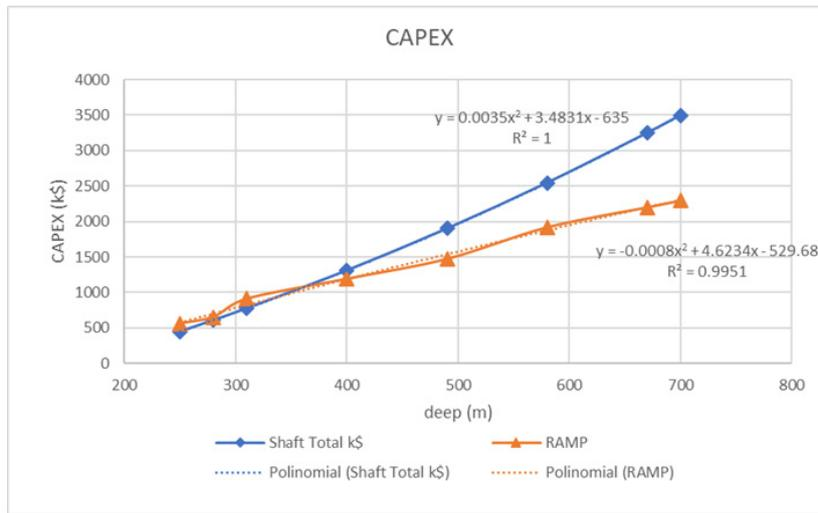
Figure 1. Capex for Ramp and Shaft adjusted for report of Elevli et al. [12].
