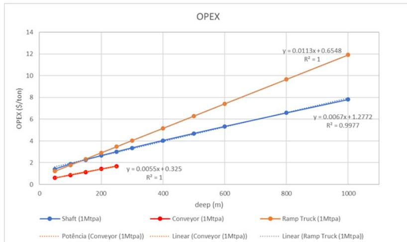
Figure 5. Opex for Ramp, Shaft and Conveyor Belt adjusted for report of Gonen et al. [10].
