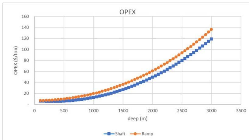
Figure 6. Average Opex for Ramp and Shaft adjusted for reports of Elevli et al. [12], Rupprecht [11], Salama [4], Gonen et al. [10].
