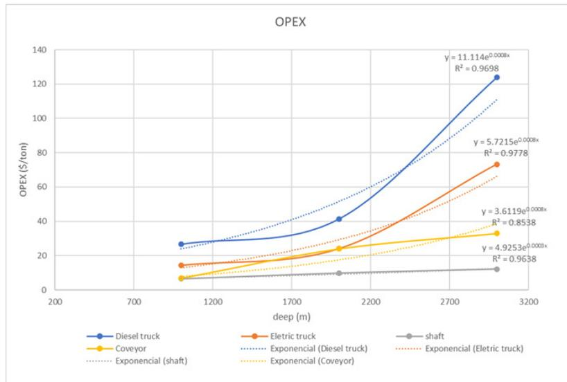
Figure 4. Opex for Ramp and Shaft adjusted for report of Salama [4].
