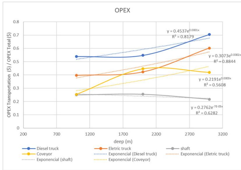
Figure 8. Relationship between transportation OpeX and Total Mining OpeX for Salama[4] data.
