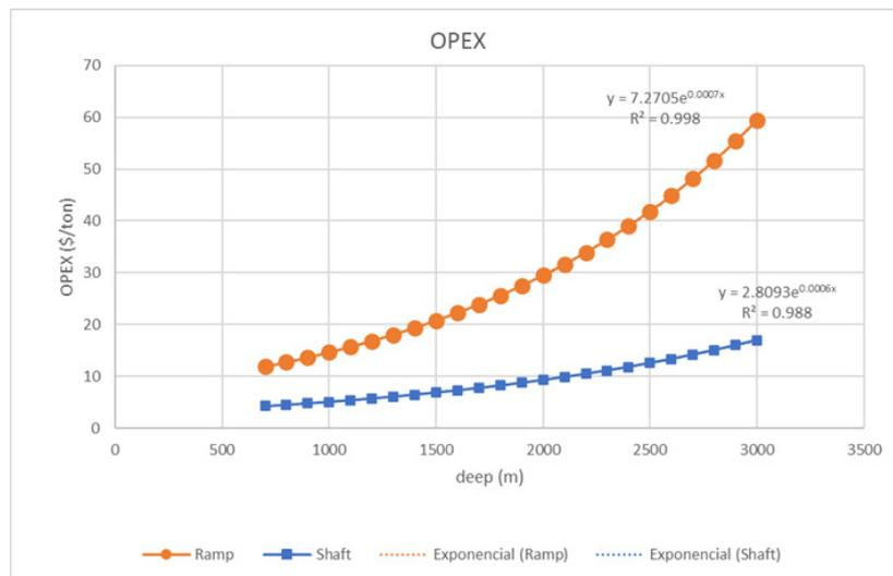
Figure 7. Average Opex for Ramp and Shaft adjusted for reports of Rupprecht [11], Salama [4], Gonen et al. [10].
