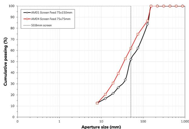
**Figure 4.** Comparative granulometric distribution for screen configurations before and after the project for the screen feed.
