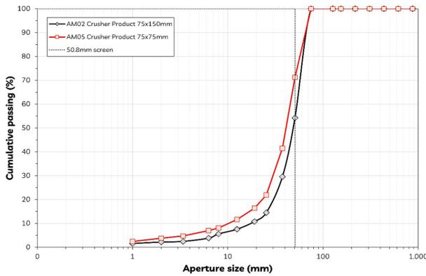
**Figure 5.** Comparative granulometric distribution for screen configurations before and after the project for the crushed material from the secondary crushers.
