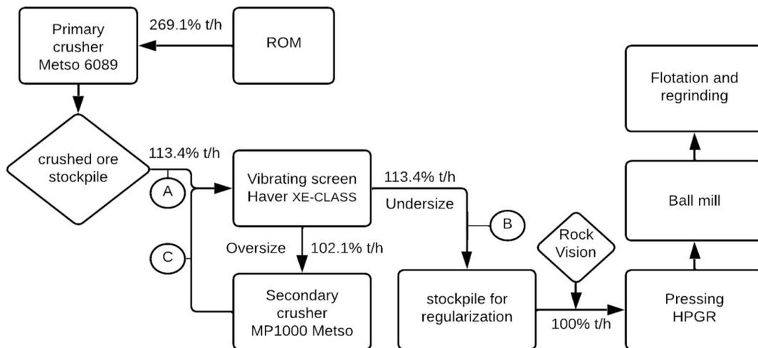
Figure 2. Processing route flowchart of Salobo's mine.
