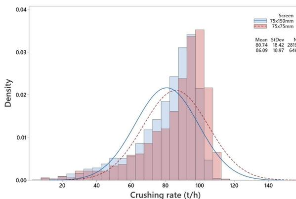
Figure 8. Histogram of secondary crushing throughput for both screen configurations.
