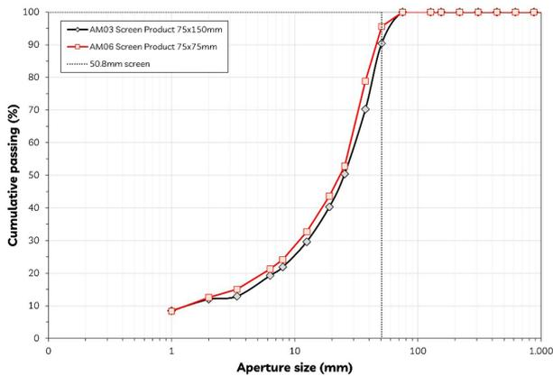
**Figure 6.** Comparative granulometric distribution for screen configurations before and after the project for the material passing through the screens.
