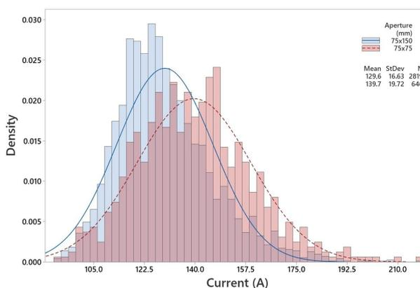
Figure 9. Histogram of total electrical current consumption for both screen configurations.
