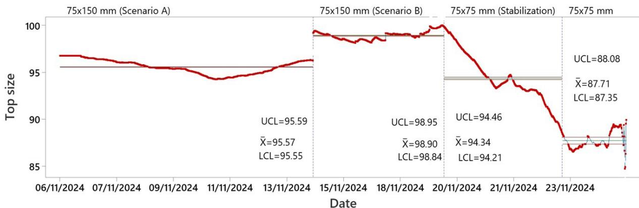
**Figure 7.** I-MR Chart of image data collected by Rock Vision regarding the top size material.
