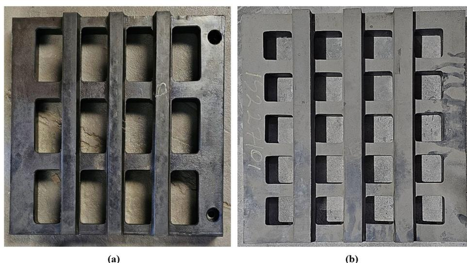
**Figure 3.** (a) 75×150 mm screen pre-design and (b) 75×75 mm screen post-design of the Haver vibrating screen in the secondary crushing circuit.
