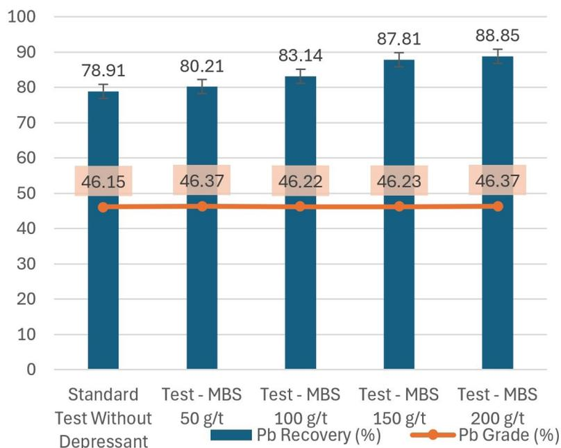
**Figure 3.** Pb Recovery and grade in the Pb concentrate as a function of MBS dosage in the Pb rougher stage.
