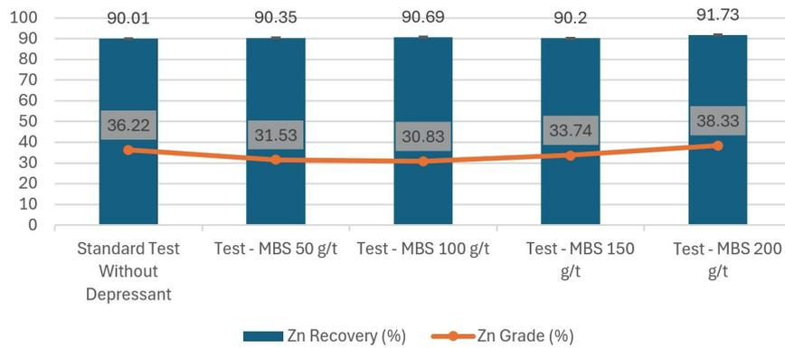
Figure 5. Zn content and recovery in the Zn concentrate as a function of MBS dosage in the sphalerite flotation stage.
