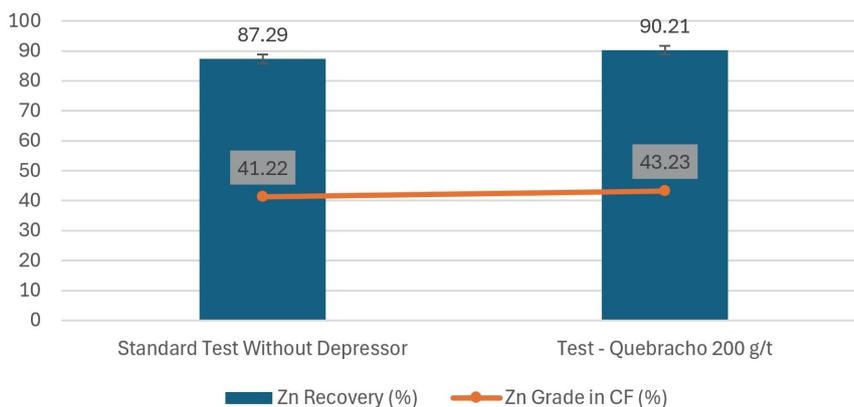
Figure 7. Zn recovery and grade in Zn concentrate with and without the use of quebracho as a depressant.
