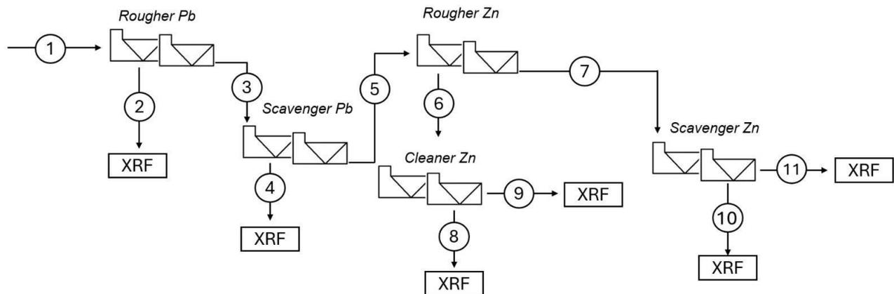
**Figure 2.** Flotation Test Flowchart. **Legend:** (1) Feed; (2) Pb Rougher Concentrate; (3) Pb Rougher Tailings; (4) Pb Scavenger Concentrate; (5) Pb Scavenger Tailings; (6) Zn Rougher Concentrate; (7) Zn Rougher Tailings; (8) Zn Cleaner Concentrate; (9) Zn Cleaner Tailings; (10) Zn Scavenger Concentrate; (11) Zn Scavenger Tailings. XRF – Chemical analysis via X-ray Fluorescence Spectroscopy.
