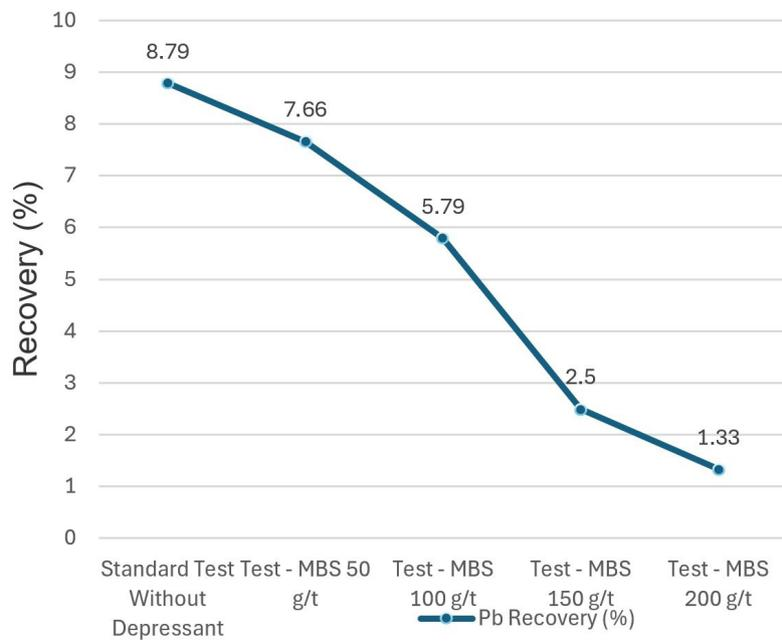
Figure 4. Pb recovery in sphalerite flotation stage as a function of MBS dosage.
