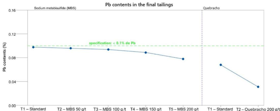
Figure 8. Pb grades in the final tailings as a function of MBS and quebracho dosages.
