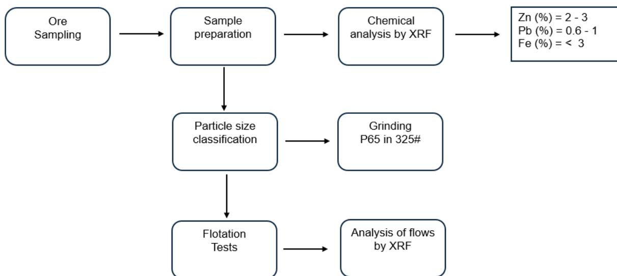
**Figure 1.** Flowchart of the Mineralogical and Particle Size Characterization Tests.
