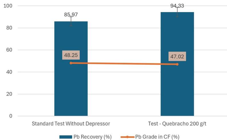
Figure 6. Pb recovery and grade in Pb concentrate with and without the use of quebracho as a depressant.
