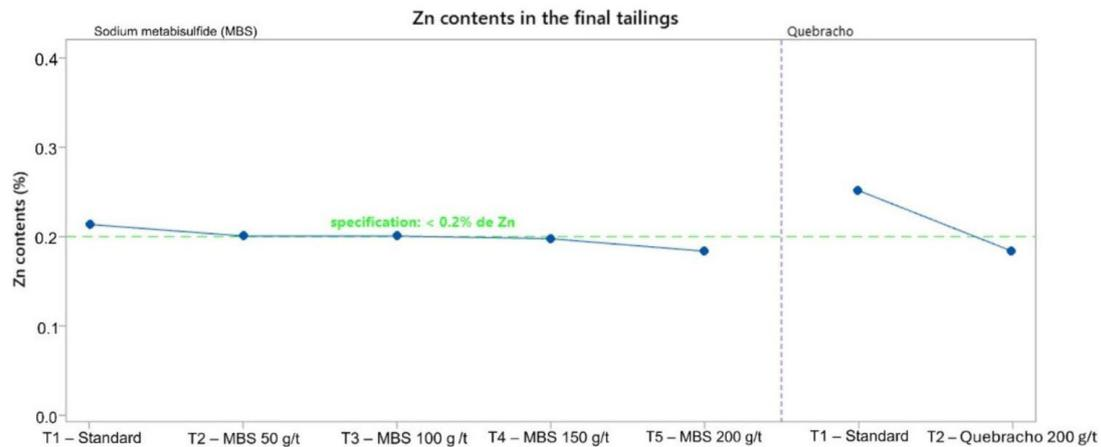
Figure 9. Zn grades in the final tailings as a function of MBS and quebracho dosages.
