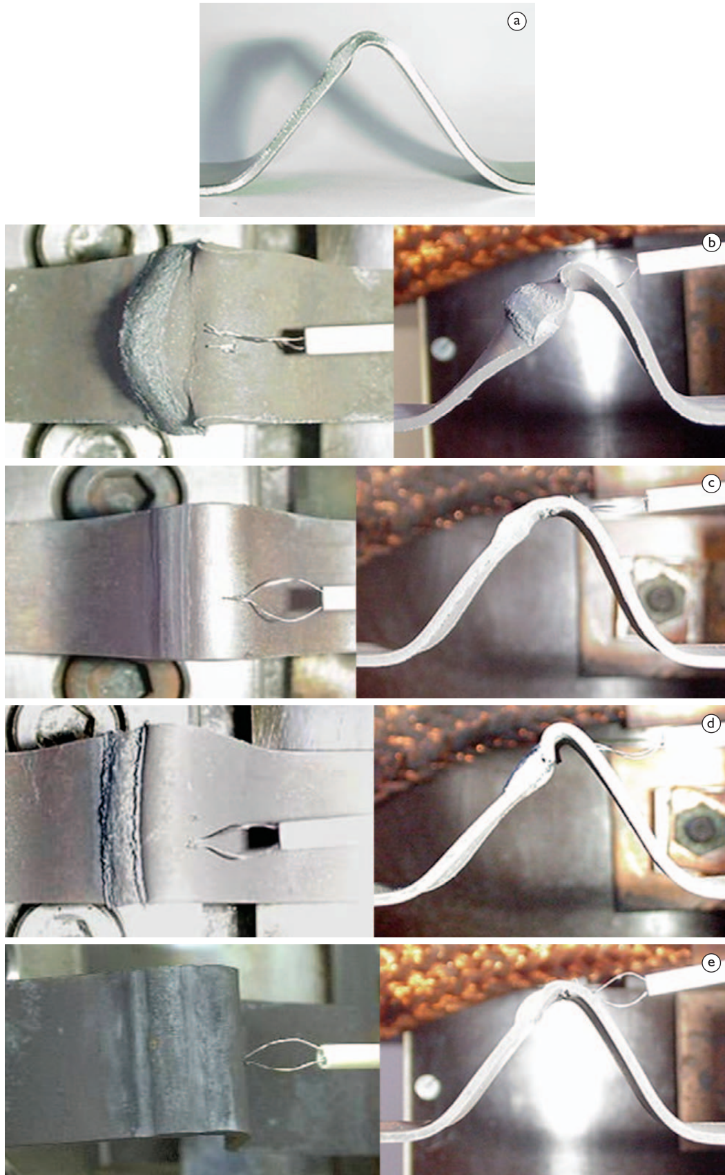
Figure 7. Sample shape at the end of the test for different base/filler metals: a) initial shape; b) K41X+307Si; c) K41X+430LNb; d) K44X+307Si; and e) K44X+430LNb.
