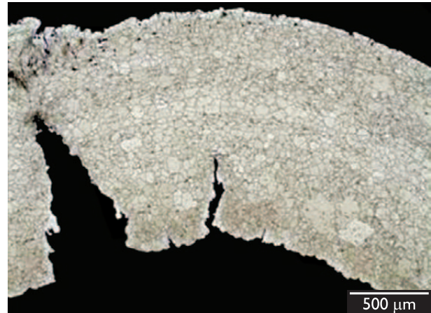
Figure 8. Initial microstructure of the weld seams – K44X MAG welding and Laser welding.
