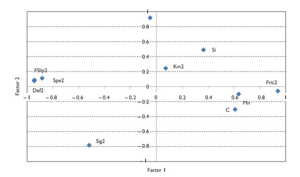
**Figure 1.** Results of the principal components analysis determined from F2 stand rolling data. Legend: C, carbon content; Mn, manganese content; Si, silicon content; T2, rolling temperature; Def2, strain degree, Km2, length of strip processed up to that moment by the work rolls; FSlip2, forward slip; Sig2, hot strength; and Fric2, friction coefficient.
