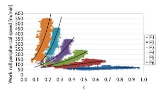
Figure 5. Work roll peripherical speed in function of strain degree  $\epsilon$  for the six rolling stands of the finishing mill.
