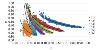
Figure 2. Friction coefficient  $\mu$  in function of strain degree  $\epsilon$  for the six rolling stands of the finishing mill.
