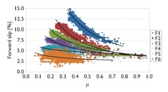
Figure 4. Forward slip in function of friction coefficient  $\mu$  for the six rolling stands of the finishing mill.
