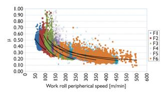
Figure 3. Friction coefficient  $\mu$  in function of work roll peripherical speed for the six rolling stands of the finishing mill.
